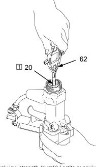
Apply low-strength (purple) Loctite or equivalent to needle shaft threads
